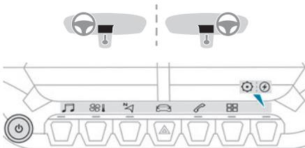
Use the buttons arranged below the touch screen to access the menus, then press the virtual buttons on the touch screen.
