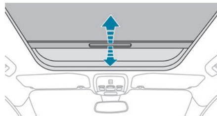
► To open/close the blind, take it by its handle and pull it backwards/forwards to the required position.
