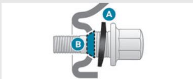
If the vehicle is fitted with alloy wheels, the washers **A** do not make contact with the steel or "space-saver" type spare wheel. The wheel is held in place by the conical contact surface **B** of each bolt.
