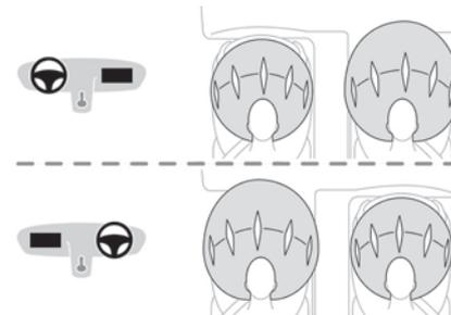
This system protects the driver and front passenger in the event of a serious front impact, limiting the risk of head and chest injury.
