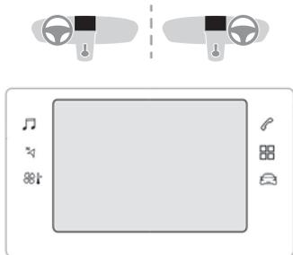
Use the buttons arranged around the touch screen to access the menus, then press the virtual buttons on the touch screen.
