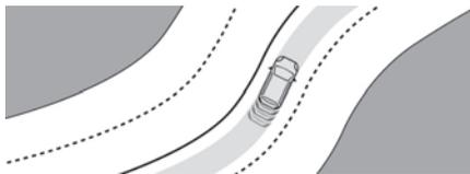
The system identifies the limits of the traffic lane and steers the vehicle inside this lane to maintain it in the lateral position chosen by the driver.
