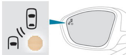
The warning is given by a fixed warning lamp that appears in the door mirror on the side in question:
