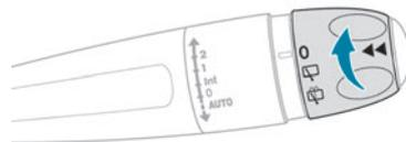
► Turn the ring to align the desired symbol with the marking.
