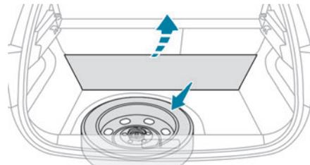
The spare wheel is stored under the boot carpet. To access the spare wheel, first refer to the **Tool kit** section.
