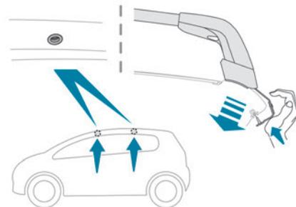
You must only attach the transverse bars to the four fixing points located on the roof frame. These points are concealed by the vehicle doors when the doors are closed.
