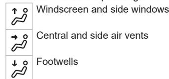
The lighting of the button indicates that air is being blown in the specified direction.
