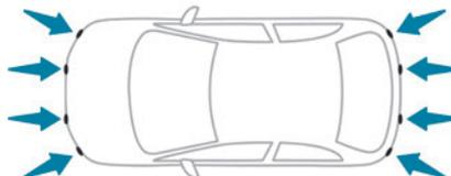
This system detects and signals the proximity of obstacles (e.g. pedestrian, vehicle, tree, barrier) using sensors located in the bumper.
