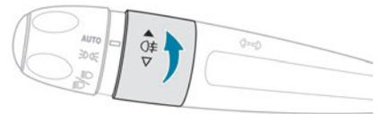
► Rotate the ring forwards/backwards to turn it on/off.
