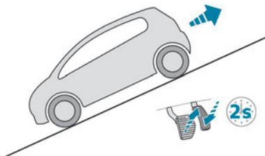
**Facing downhill, with the vehicle stationary and reverse gear engaged, the vehicle is held for a short time when the driver releases the brake pedal.**
