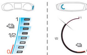
The traction battery's actual charge level and the remaining range are displayed continuously when the vehicle is started.
