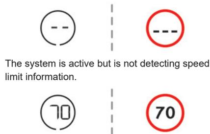
On detecting speed limit information, the system displays the value.
