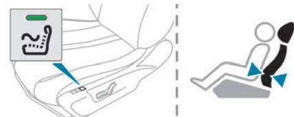
This function provides lumbar massage; it only operates when the engine is running as well as in STOP mode of the Stop & Start system.
