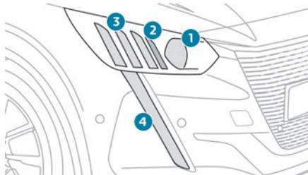
1. Dipped beam headlamps / Main beam headlamps
