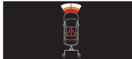
**i** The rear parking sensors system will be deactivated automatically if a trailer or bicycle carrier is connected to a towing device installed in accordance with the manufacturer's recommendations. In this case, the outline of a trailer is displayed at the rear of the image of the vehicle.
