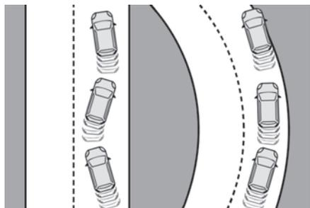
**i** The system assesses the driver's level of alertness, fatigue and distraction by identifying trajectory changes in relation to the lane markings.
