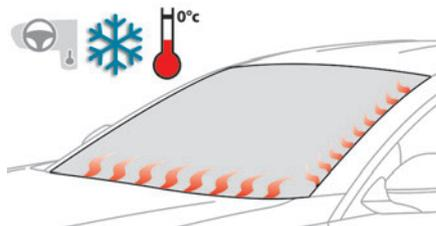
In cold weather, this system heats the bottom of the windscreen, as well as the area alongside the left-hand windscreen pillar. Without changing the settings for the air conditioning system, it allows faster release of the windscreen wiper blades when they are frozen to the windscreen and helps avoid
