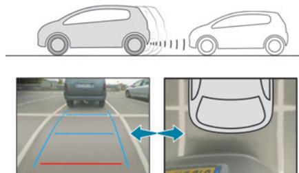
This mode is activated by default. Using sensors in the rear bumper, the automatic view changes from the rear view (standard) to the view from above (zoom) as an obstacle is approached at the level of the red line (less than 30 cm) during a manoeuvre.
