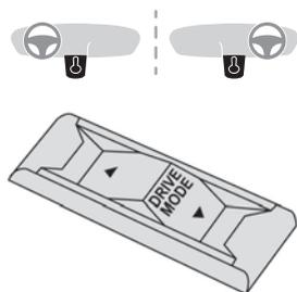
► Press the control to display the modes on the instrument panel, and depending on version, on the screen with PEUGEOT Connect Nav.
