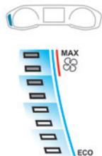
The gauge shows the consumption of the traction battery's electrical energy by the thermal comfort devices in the passenger compartment. With a digital instrument panel, the gauge only appears in **"Personal"** mode.
