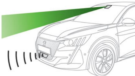
The vehicle has a multifunction camera located at the top of the windscreen and, depending on version, a radar located in the front bumper.
