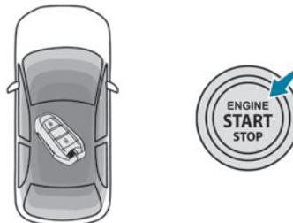
With the electronic key in the passenger compartment, pressing the **"START/STOP"** button, **without depressing any of the pedals**, allows the ignition to be switched on without starting the engine.
