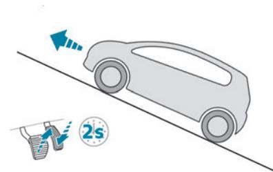
**Facing uphill, with the vehicle stationary, the vehicle is held for a short time when the driver releases the brake pedal:**
