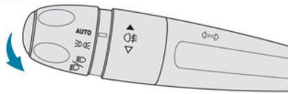
► Pull the lighting control stalk to switch between dipped and main beam headlamps. In lamps off or "AUTO" modes, depending on version, and in sidelamps mode, pull the lighting control stalk to switch the main beam headlamps on directly ("headlamp flash").
