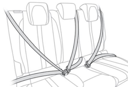
Each of the rear seats has a three-point seat belt with inertia reel.
