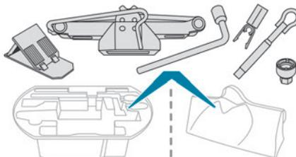
! These tools are specific to the vehicle and may vary according to the level of equipment.
