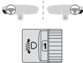
To avoid dazzling other road users, the height of these headlamp beams must be adjusted according to the load in the vehicle.
