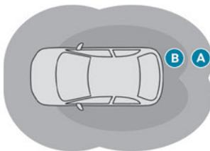
**Zone A:** automatic locking on moving away from the vehicle (about 2 metres from the vehicle).
