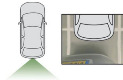
The camera records the vehicle's surroundings during the manoeuvre in order to create a view from above the rear of the vehicle in its near surroundings, allowing the vehicle to be manoeuvred around nearby obstacles.
