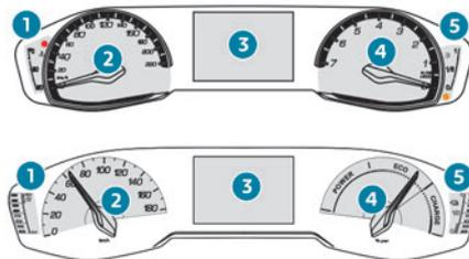
1. Coolant temperature indicator (°C) (Petrol or Diesel)
