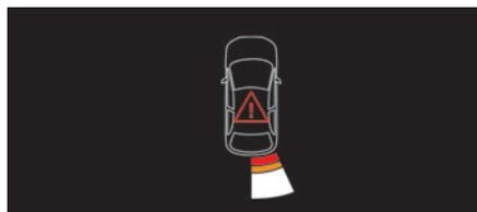
This supplements the audible signal by displaying bars on the screen whose location represents the distance between the obstacle and the vehicle (white: more distant, orange: close, red: very close).
