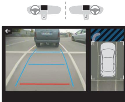
The screen is divided into two parts with a contextual view and a view from above the vehicle in its close surroundings. The parking sensors supplement the information on the view from above the vehicle. Various contextual views may be displayed:
