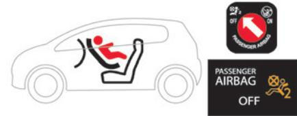
! The front passenger airbag must be deactivated before installing a rearward facing child seat. Otherwise, **the child risks being seriously injured or killed if the airbag is deployed.**
