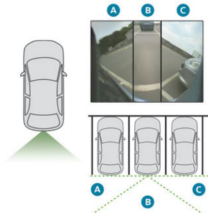
The 180° view facilitates reversing out of a parking space, making it possible to see the approach of vehicles, pedestrians and cyclists. This view is not recommended for carrying out a complete manoeuvre.
