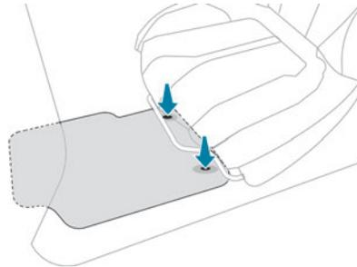
When fitting it on the driver's side, only use the mountings present on the carpet (a "click" indicates proper locking). The other mats are simply laid over the carpet.
