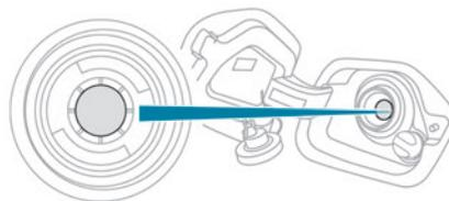
When a petrol filler nozzle is introduced into the fuel filler neck of a Diesel vehicle, it comes into contact with the flap. The system remains closed and prevents filling.
