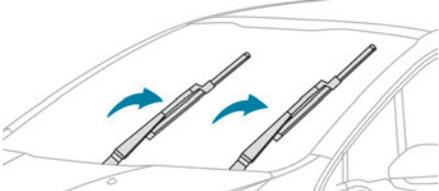
Operating the wiper control stalk immediately after switching off the ignition will place the wiper blades in a vertical position.
