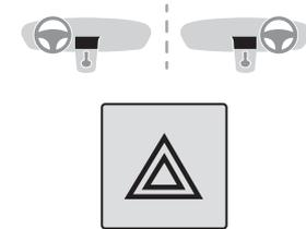
► Pressing this red button causes all the direction indicators to flash. They can work with the ignition switched off.
