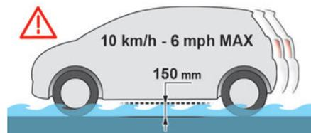
If the vehicle absolutely must drive through a flooded section of road:
